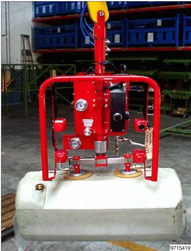
Manipulator with adjustable suction cups tooling (Venturi) for gripping and handling tanks.
