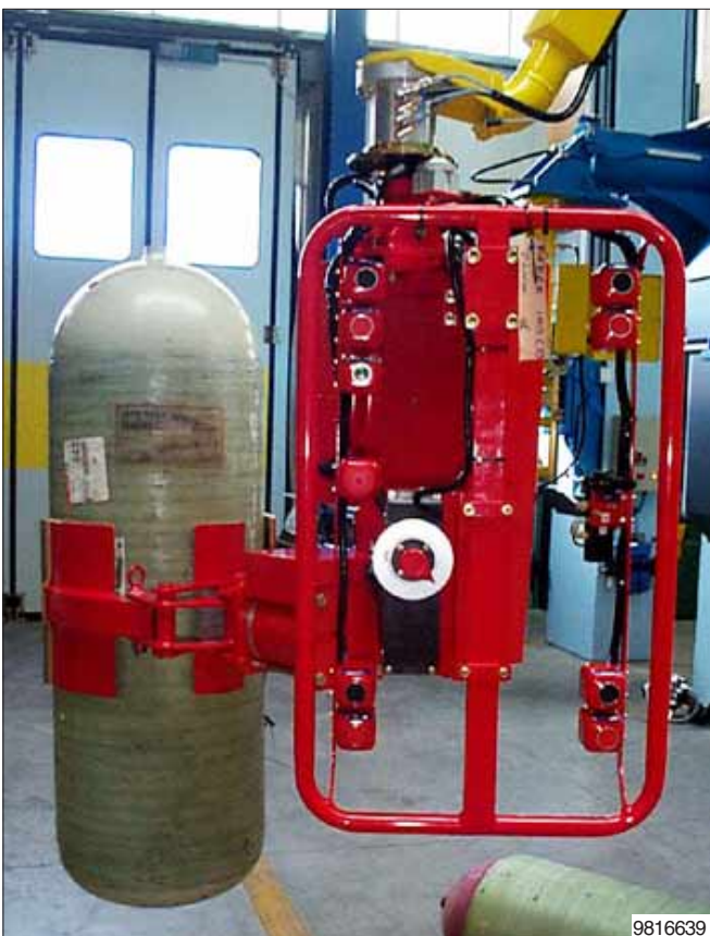
Manipulator with pneumatic tooling for gripping and inclination of cylinders having different dimensions.
