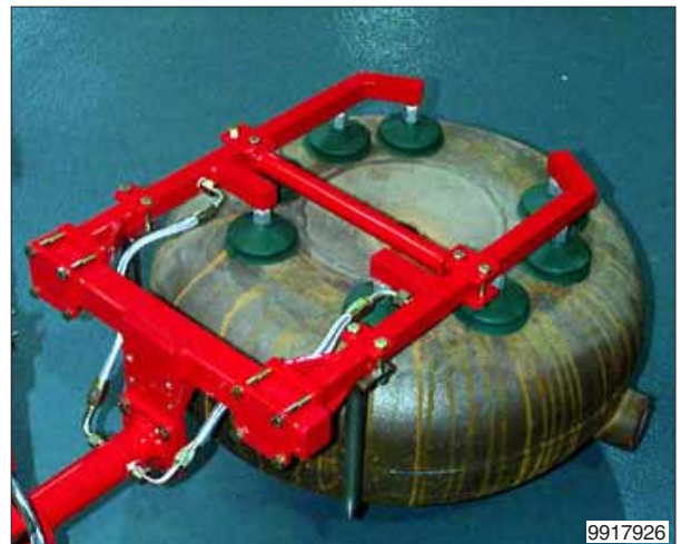
Manipulator with suction cup tooling (Venturi) for gripping and manual rotation of tanks.
