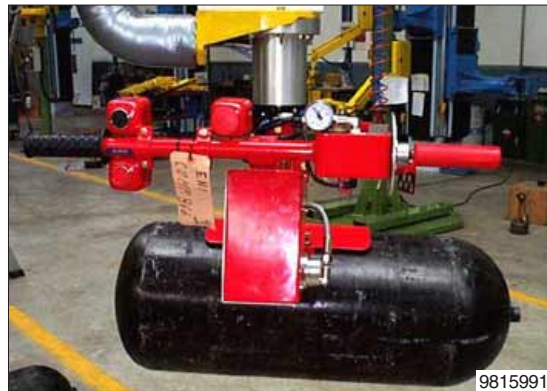
Manipulator with suction cup tooling (Venturi) for gripping and releasing the tanks into the car.
